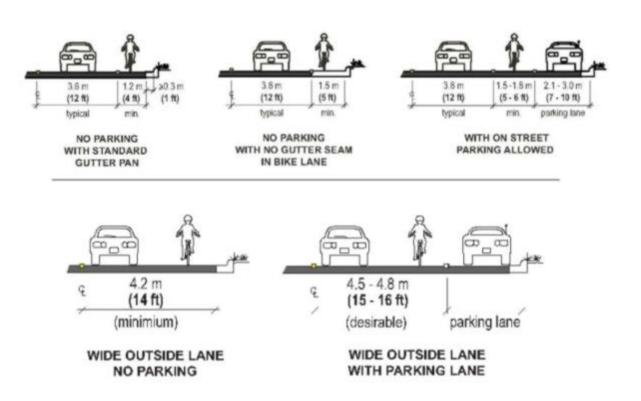
Figure 4-6: Bicycle Lane with No Parking and Standard Gutter Plan
