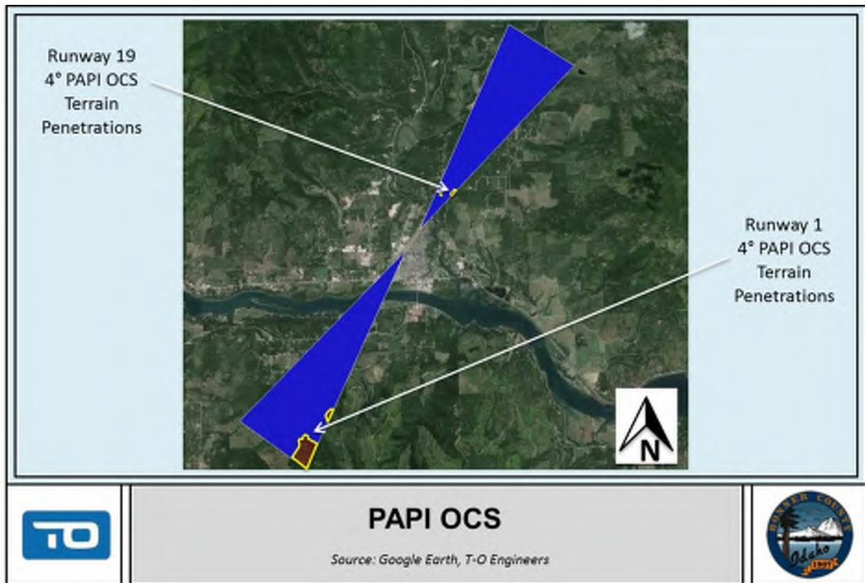
**Recommendations:** Initial feasibility analysis for PAPIs on both runway ends indicates the installation of the approach path system might be feasible. Mitigation via use of baffling or by restricting lateral coverage may be an option. Further coordination and verification with the FAA is recommended to conduct additional analysis.
