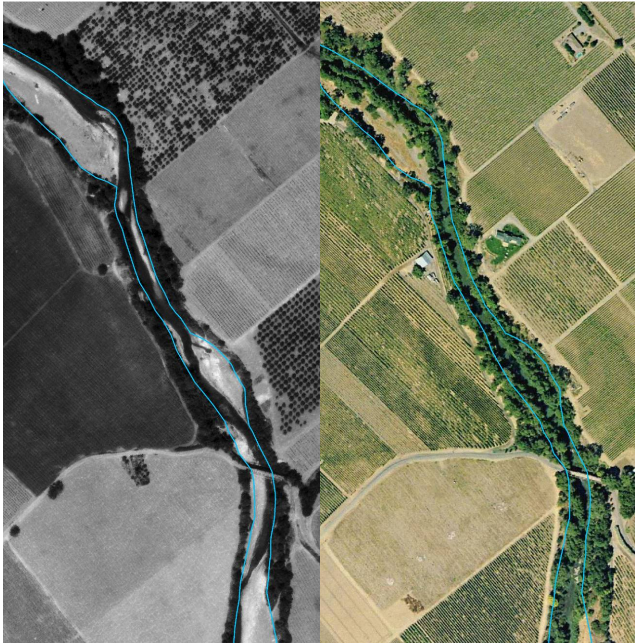
Figure 17: Example of vegetative narrowing of channel corridor near Lambert Bridge (RM 6.6). Lambert Bridge is seen at lower right of each frame. Dry Creek flow is from top to bottom. Left frame is from 1976, right frame is from 2004. Light blue line is estimated limit of active fluvial features in 1976.
