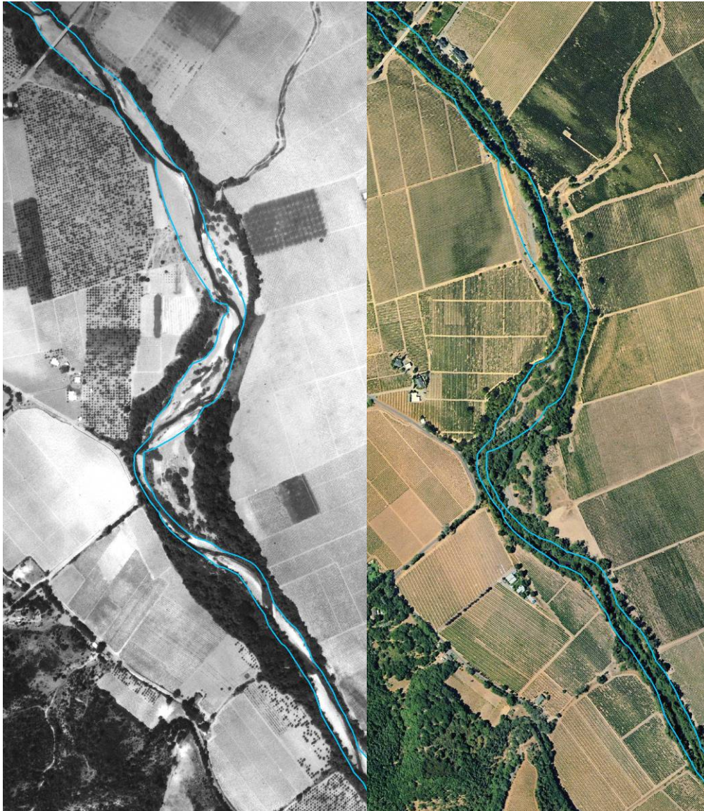
Figure 15: Example of vegetative encroachment near Yoakim Bridge. Yoakim Bridge (RM 10.7) is seen at upper left of each frame. Dry Creek flow is from top to bottom of each frame. Left frame is from 1976, right frame is from 2004. Light blue line is estimated limit of active fluvial features in 1976.
