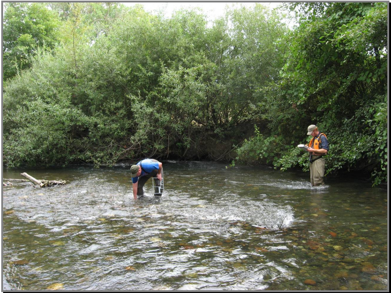
Photograph 2. Field crew conducting Wolman pebble count.
