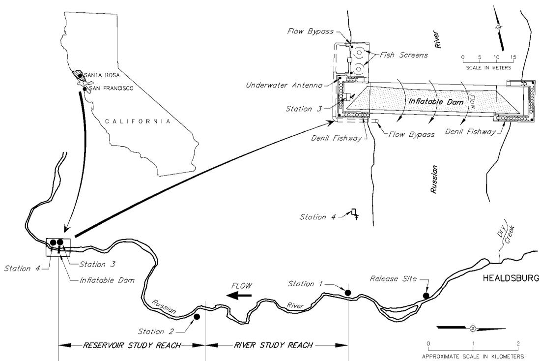
FIGURE 1.—Map of the study area showing the free-flowing (river) and impounded (reservoir) reaches of the Russian River, California, and detail of Mirabel Dam. Stations 1–4 represent data-logging radiotelemetry receiver sites. Underwater antenna locations in the dam forebay are shown as shaded circles.
