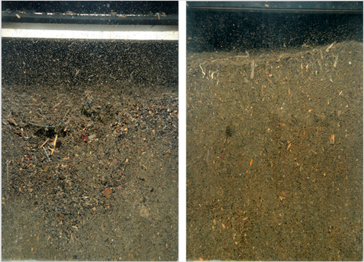
Figure 3-11. These profile images from Station 1-19 (left) and 1-32 (right) are typical of the locations where sediment-oxygen demand was so high that no detectable aRPD could be measured. Scale: width of each profile image = 14.4 cm.
