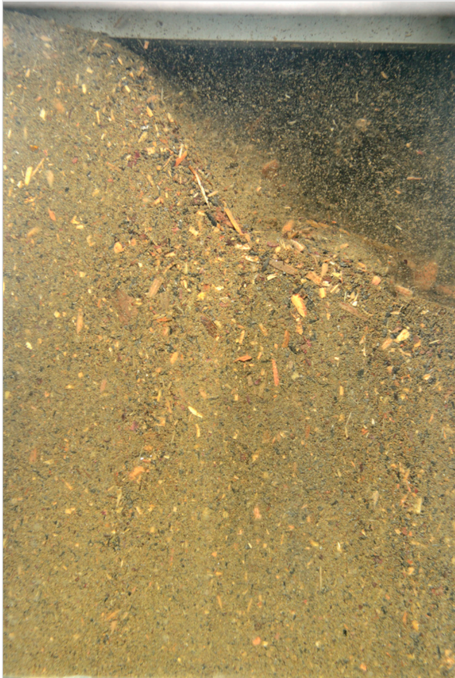
Figure 3-9. This profile image from Station 1-31 had an unusually high boundary roughness value (9.8 cm) due to a sloping bottom. Scale: width of image = 14.4 cm.
