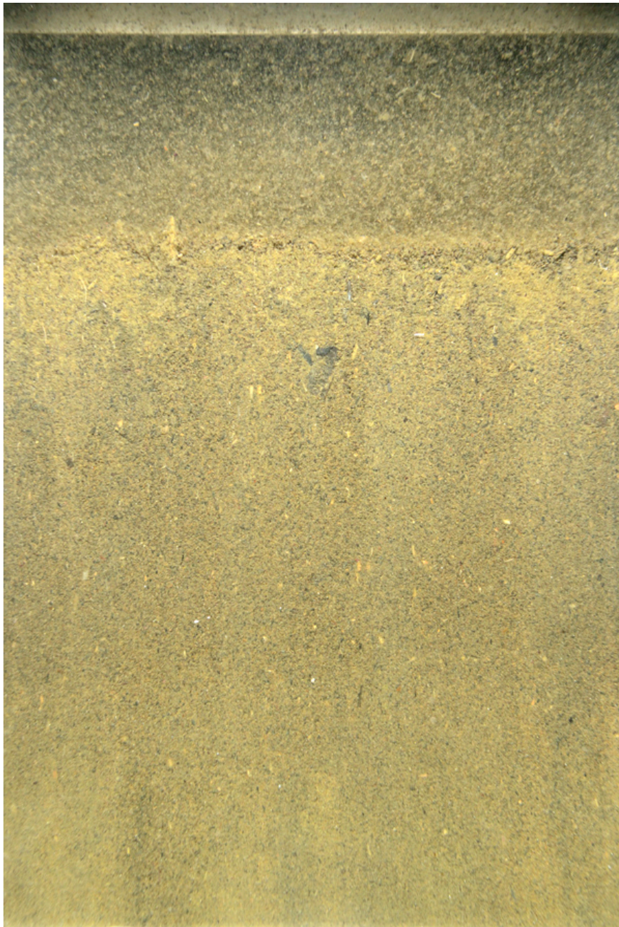
Figure 3-2. The higher fraction of very fine sand mixed in with wood fibers and silt-clay sediments was typical of the stations sampled closest to the shoreline of the former APC site. Scale: width of profile image = 14.4 cm.
