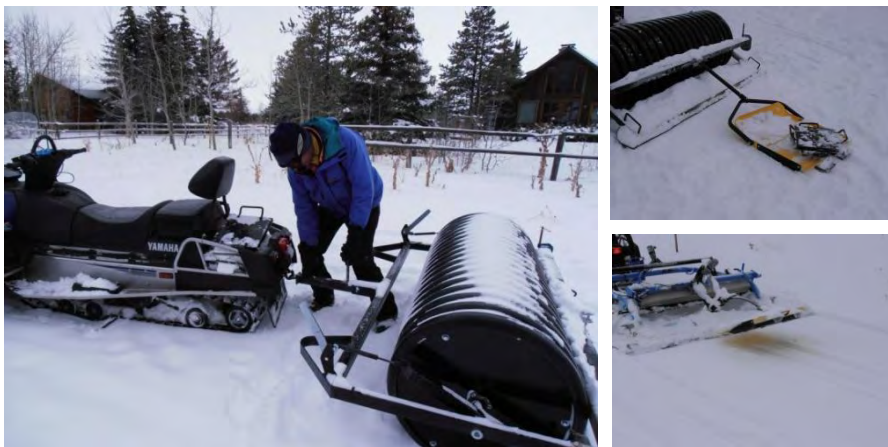
Figure 20 – Small scale nordic grooming equipment – roller, track setter and ginzugroomer
