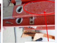
Cracked Fiberglass Rail
